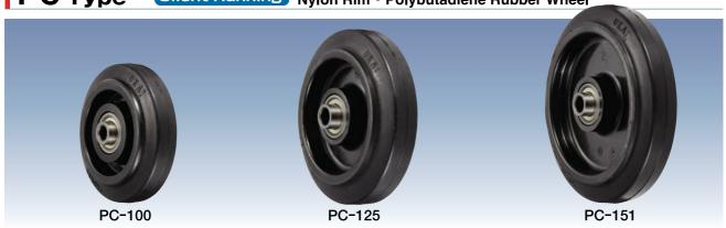
Unit: mm Boss Width **Load Capacity** Tire Shaft Weight Size Width Diameter (g) Steel В R D kg Compatible Radial **Model Number** Caster  $(\circ)$ Bearing (daN) (kgf) 6200ZZL 100 PC-100 120 122.4 42 32 10 270 PCJC 125 PC-125 150 153.0 53 38 12 6201ZZL 410 PCKC, PCKE **PCJCS** 150 PC-151 180 183.6 53 38 12 6201ZZL 500
